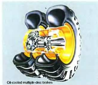
Oil-cooled multiple-disc brakes
